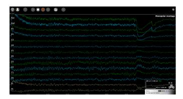
NeoRec cap is intended to record EEG and 3D acceleration events to files of different formats (EDF+ 16 bit, BDF+ 24 bit, GDF 32 bit) or transmit it on-line via stream LSL (Lab Streaming Layer) for analyze by third-party software as MATLAB / EEGLAB, OpenViBE etc.
